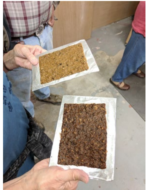
samples of mushroom pulp after being formed into paper.
