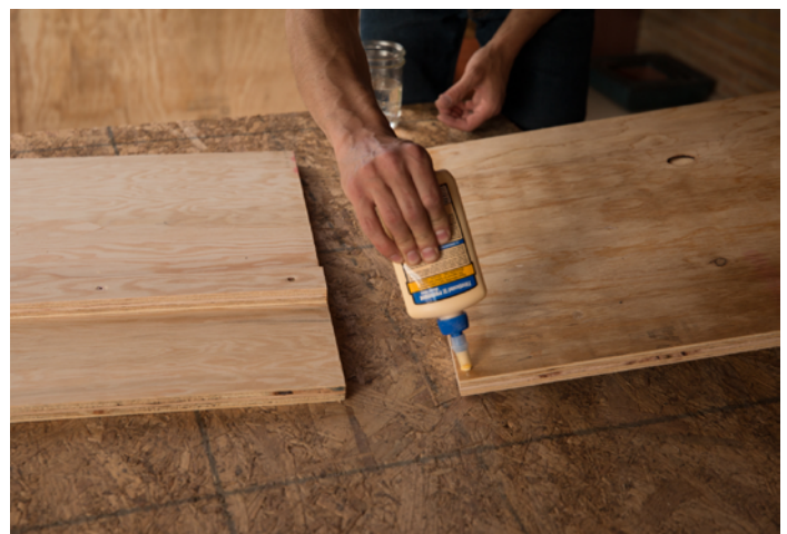
The piece on the left shows a strip that prevents the air filter from falling into the box. Ben is applying glue to the piece on the right to begin the process of assembling the box.
