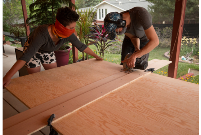
Ben and Mercedes making cuts with a homemade fence and a circular saw... a table saw would be so much better!
