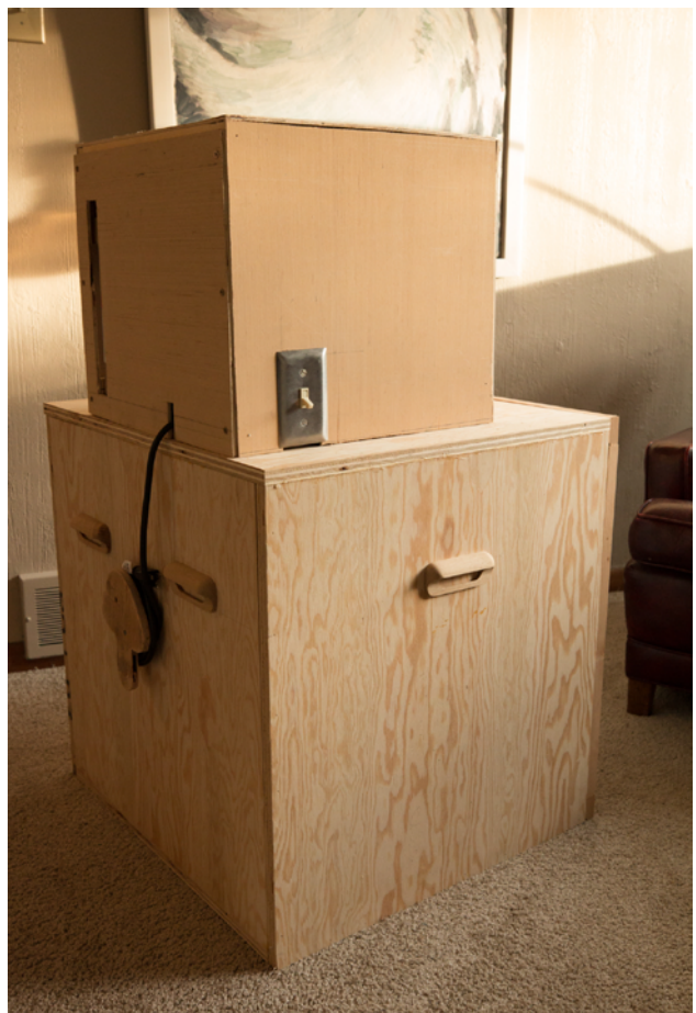
We mounted the switch plate to the outside of the box and also installed handles for ease of moving around.
