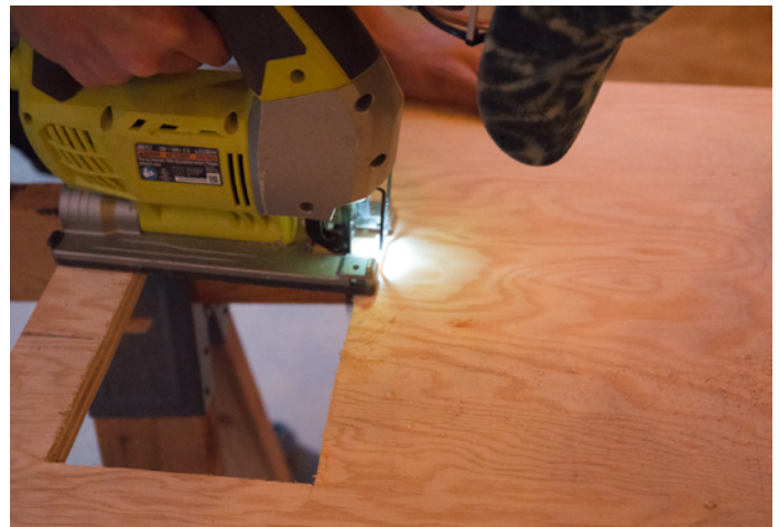
Measure the blower to determine how big of a hole you need, then use a jig saw to cut out the area.
